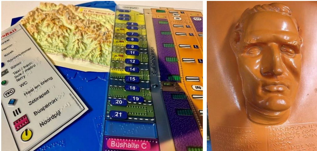
Figure 7.10 Examples of vacuum forming used for maps and even a portrait of Louis Braille. (Photos A.M. Conefrey)
